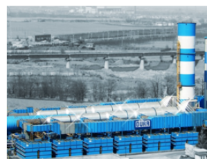
Dürr mine mouth methane capture equipment in Shanxi, China
